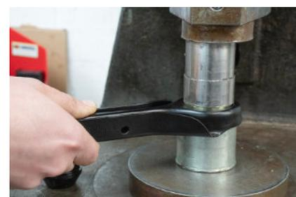
Figure 2. Press in the outer sleeve.
