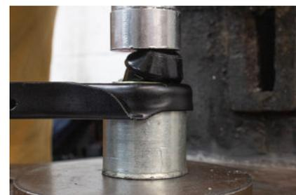
Figure 3. Bush pressed at an angle.
